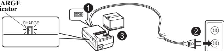
If the CHARGE indicator does not light, check that the connections (1), (2), and (3) are firmly made.
